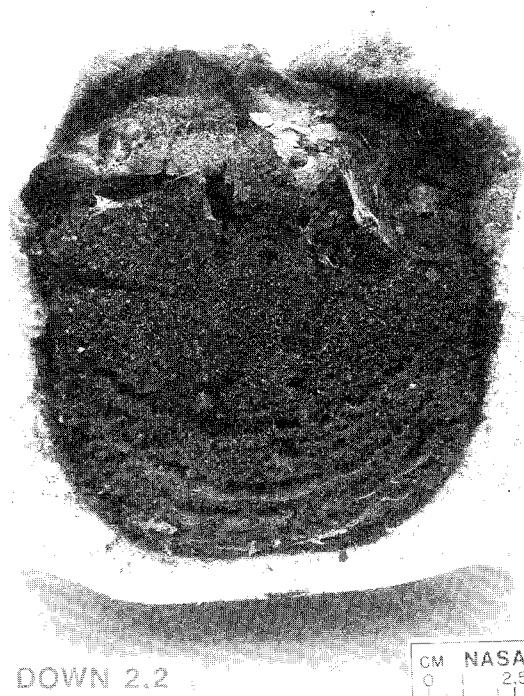
Fig. 11 Photograph showing a cut sample of burnt foam from a downward smoldering experiment.
